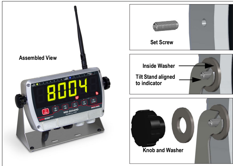
Figure 2-12. Install Tilt Stand
